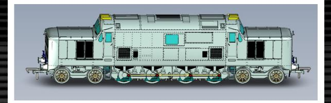
Progress on the Fell is also moving along steadily. Here are the final CAD drawings with the additional full connecting rod. All you will need to do, if you do want the full rod, is remove the two rods and replace it with the full rod.
